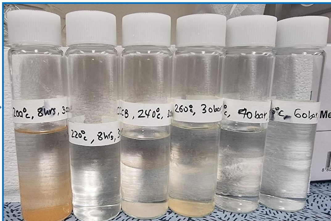
Product separation using ethyl acetate as organic solvent
